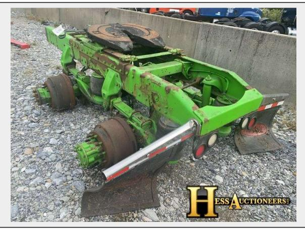
TRUCK PART TYPE SUSPENSION CUT OFF
