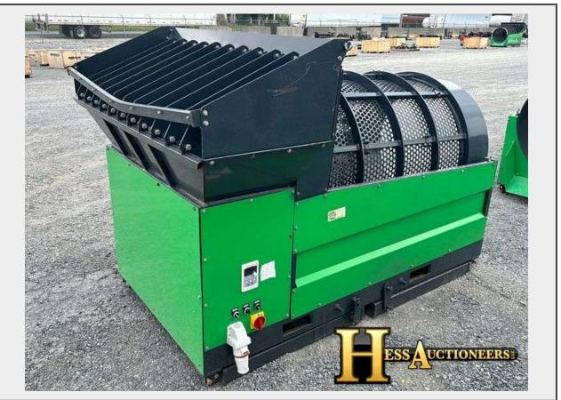
Model GF480 ROTARY DRUM Attachment Type SCREENER Detailed Category SKID STEER ATTACHMENT Notes diameter 48'' capacity approximately 20-40 tons per hour Stock # 87825
