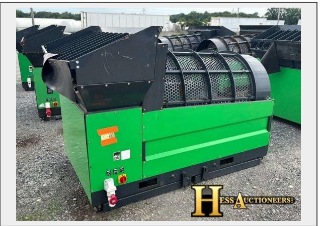
Model GF480 ROTARY DRUM Attachment Type SCREENER Detailed Category SKID STEER ATTACHMENT Notes diameter 48'' capacity approximately 20-40 tons per hour Stock # 87813
