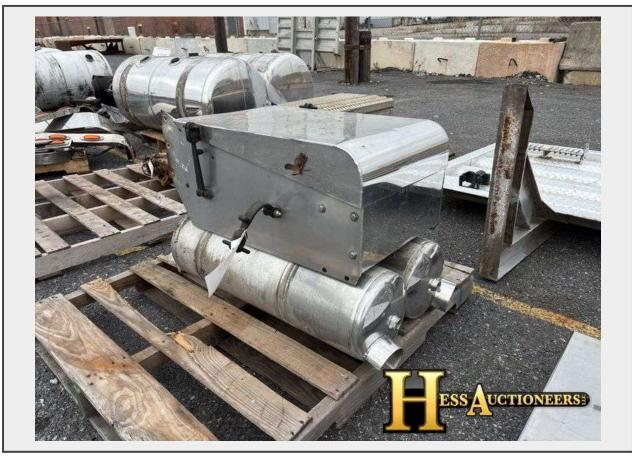
TRUCK PART TYPE AIR TANKS AND BATTERY BOX
