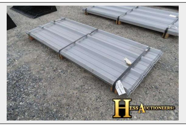
**Building Material Type** 24 GAUGE GALVANNEALED R PANELS
